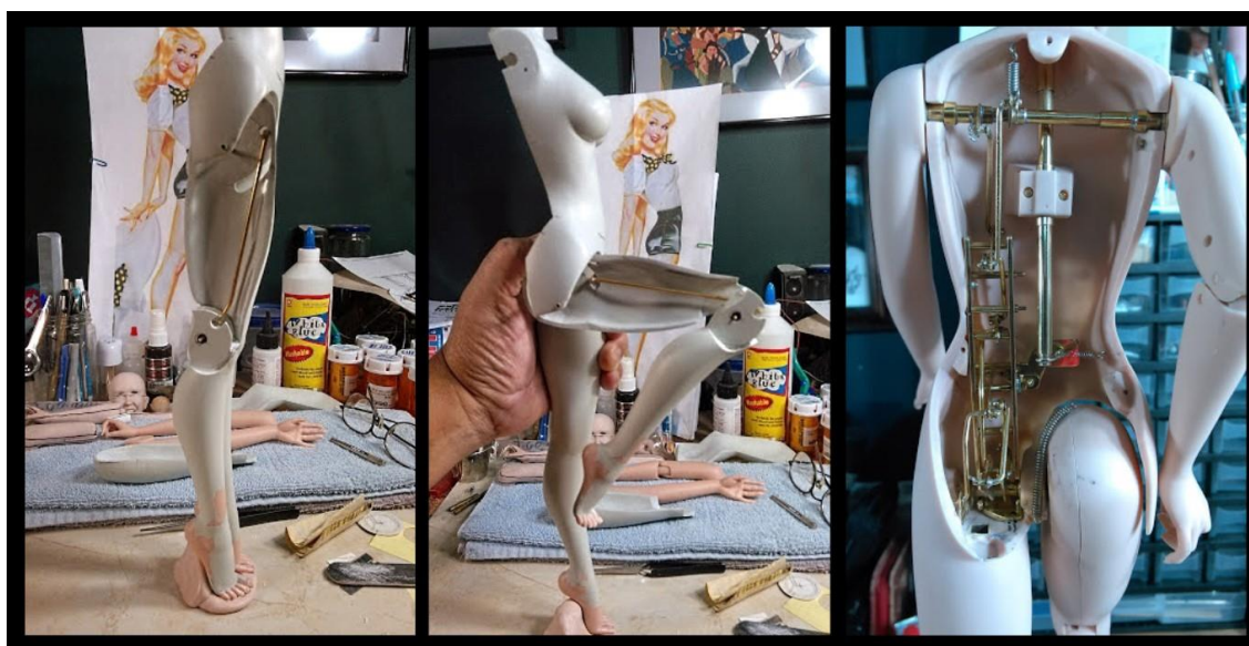
Figure 6. Inside of Marilyn Monroe automaton leg (left and middle). Inside the back of the automaton, displaying the solid brass mechanism that makes her move (right). By Joe MacPhale, 2016, resin, 19” From personal communication. Copyright by Joe MacPhale. Reprinted with permission.
