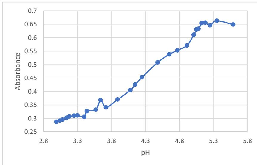
**Figure 7:** Humulone and water solution from pH 2.99 through 5.59 at 206 nm.
