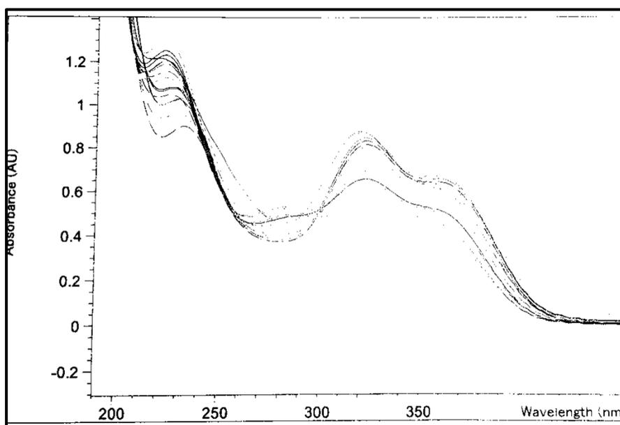
**Figure 3:** Humulone / magnesium solution separated from the spectra in Figure 1. pH values range from 3.78 to 7.18.
