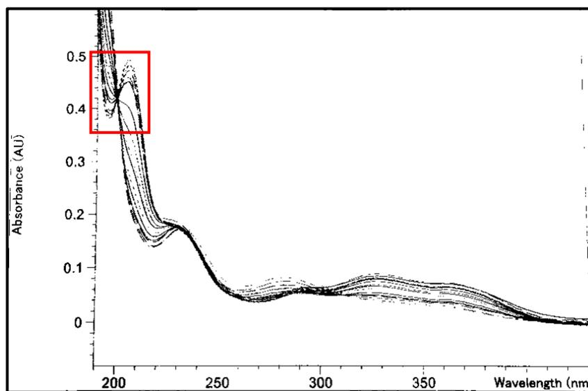
**Figure 5:** UV-vis spectra of humulone and water solution. pH values ranged from pH 2.99 to 5.59.
