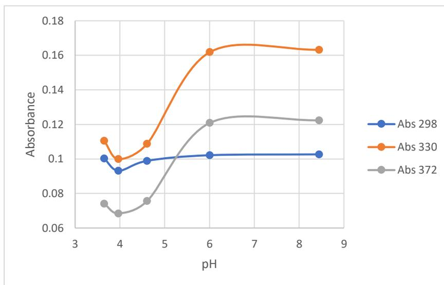
**Figure 6:** Humulone and magnesium solution from pH 3.65 through 8.45. Absorbance values collected from 298, 330 and 372 wavelengths (nm). (keep)
