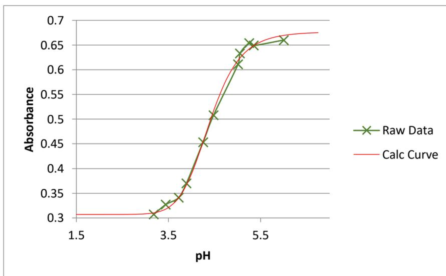
**Figure 8:** Values taken from Figure 12 to represent the sigmoidal curve. These data are overlaid with a computer-generated sigmoidal curve generated as a logistical equation.
