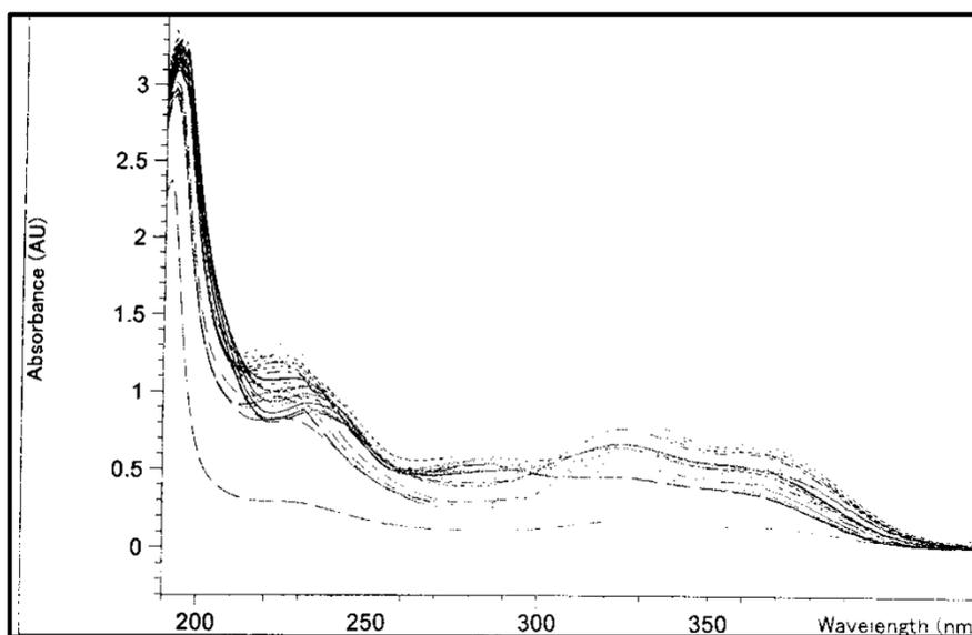
**Figure 1:** UV-vis spectra of humulone and water solution and humulone with magnesium. pH values range from 3.03 to 10.72. Spectra taken based on Procedure 2.
