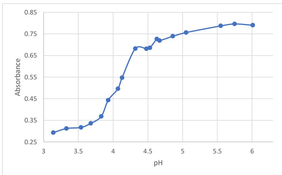
**Figure 15:** Humulone and magnesium solution from pH 3.14 through 6.01 at 206 nm. Values are from spectra taken using Procedure 1.
