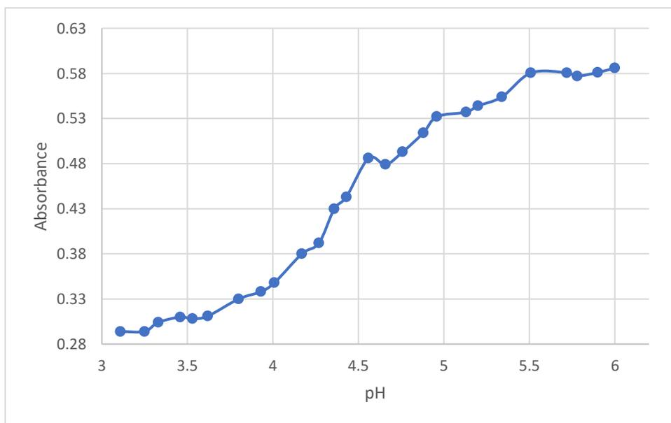
**Figure 11:** Humulone and water solution from pH 3.11 through 6.00 at 205 nm. Values are from spectra taken using Procedure 1.
