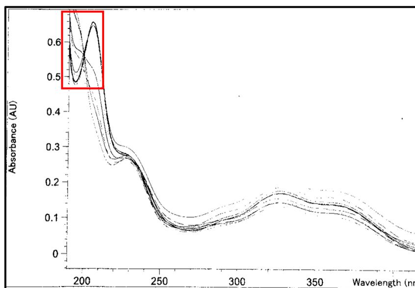
**Figure 4:** UV-vis spectra of humulone with Magnesium. pH values ranged from pH 3.06 to 6.22.
