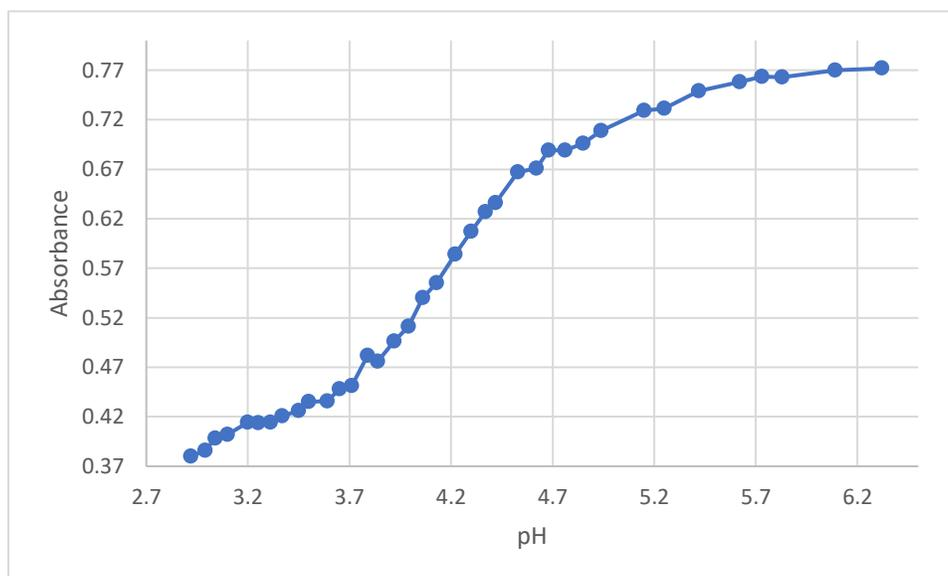
**Figure 17 :** Humulone and magnesium solution from pH 2.92 through 6.32 at 206 nm. Values are from spectra taken using Procedure 1.
