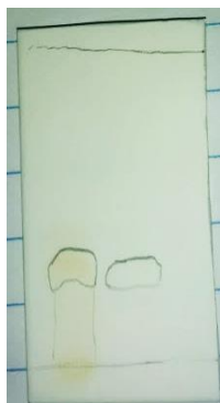
Figure 19: Image of TLC plate used for developing the Yamazen Smart Flash method. Left lane is crude cannabinoid extract, right lane is \Delta^9 -THCA obtained from an unpictured TLC plate.
