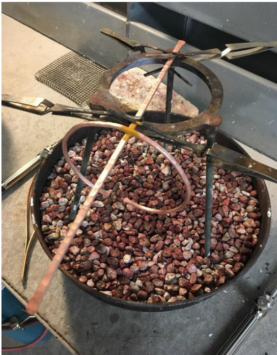
Figure 21. Hammered wire ready to be soldered, Fogarty, 2017.
