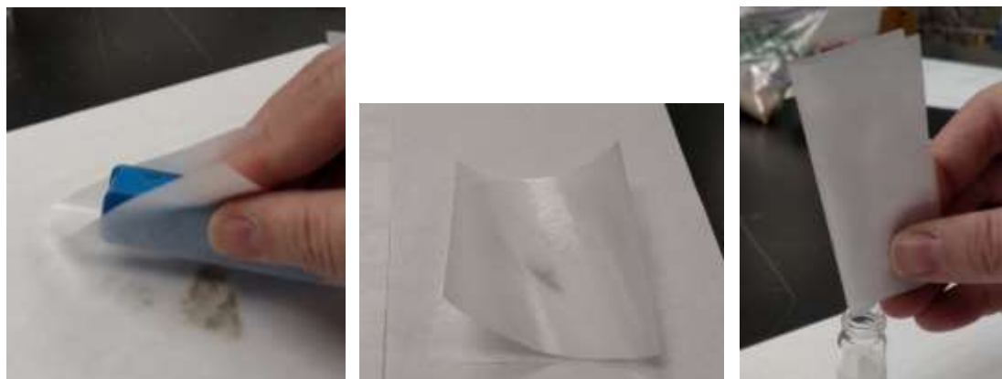
Figure 7. Images of dry separation process from left to right: Collecting magnetic material, magnet is removed leaving magnetic material on bottom sheet of weight paper, magnetic material is placed in a vial.
