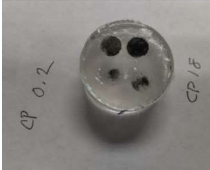
Figure 10. Grain mount in epoxy for samples CP0.2 and CP18.0 before coating in carbon.
