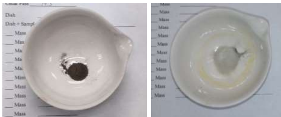
Figure 9. Sample CP18 before HCl on the left and after HCl on the right.
