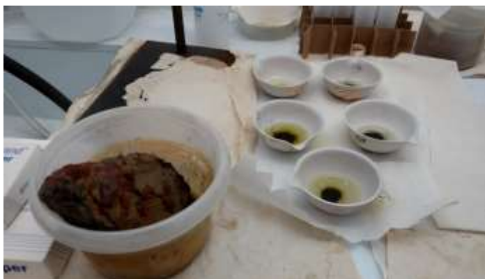
Figure 8. Samples in HCl in the fume hood.
