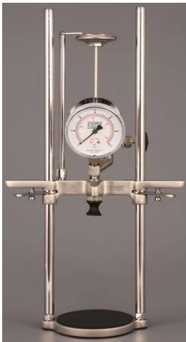
Figure 3.14: Photograph of a Zahm and Nagel CO 2 piercing device (Zahm & Nagel, n.d.)
