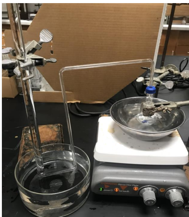
Figure 3.9: Photograph of the bubble analysis setup. The reaction was contained in a round bottom flask set inside a hot water bath. An adapter connecting a glass tube to the reaction vessel was connected to a gas collection tube that was filled with warm water
