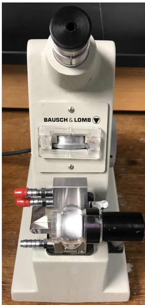
Figure 3.13: Photograph of the Bausch & Lomb ABBE-3L refractometer used to determine the refractive index and ultimately obtain the specific gravity of the wort solutions
