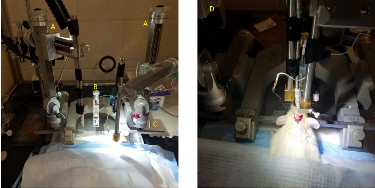
**Figure 8.** Stereotaxis apparatus example. (A) Arms contain measurement knobs (in mm) which direct probe placement into the subject. (B) Nose bar which fits over the mouth and nose to secure the subject and orient head tilt. (C) Ear bars also secure the subject and orient measurements for electrode implantation. (D) Alternate view of stereotaxis arm, which can hold electrodes for subject implantation.
